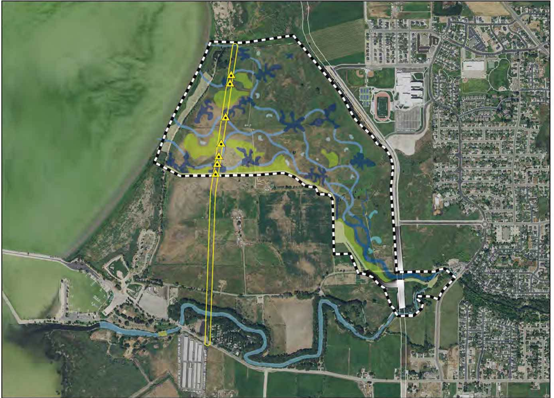
Figure 7. Map showing the location where a natural gas pipeline was surveyed in the field (triangles) and a rough location where the new pipeline will be placed (yellow outline). The new pipeline will be buried deep enough to avoid any safety issues for construction.
