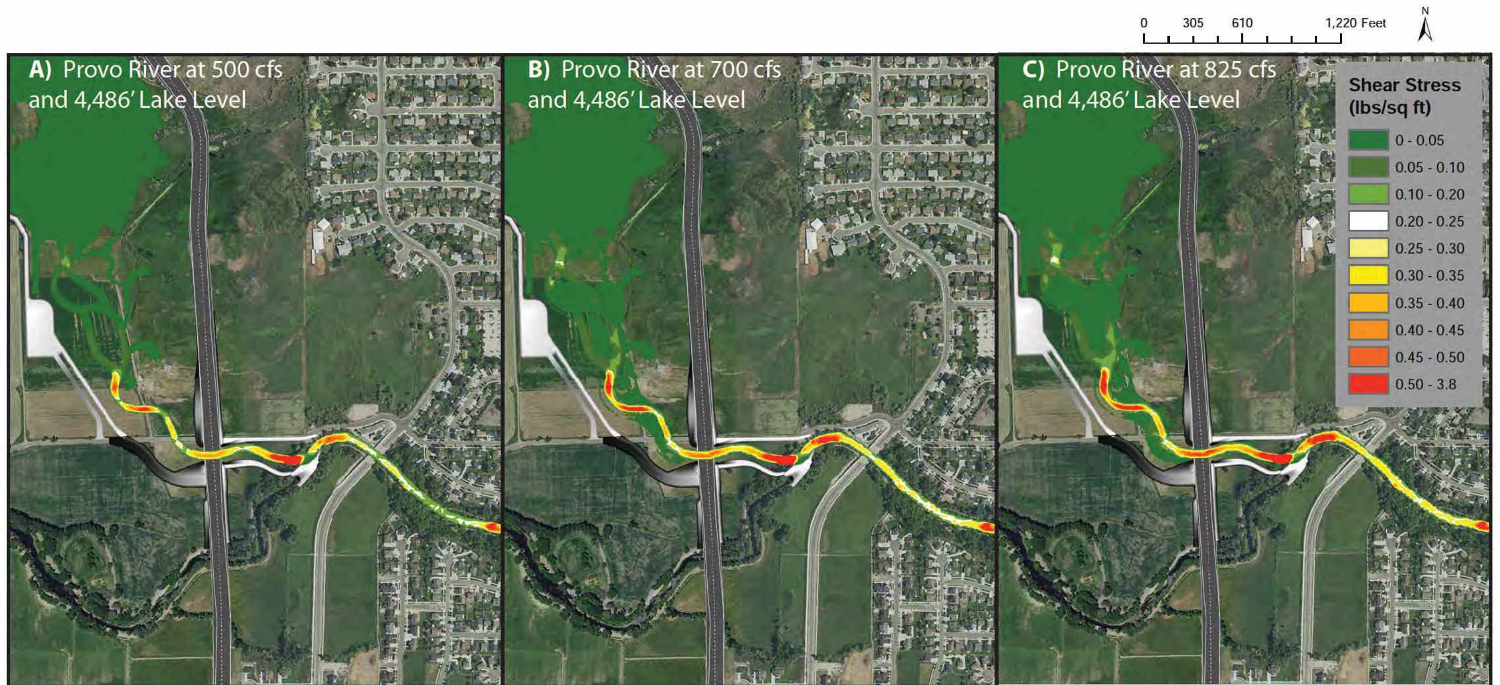
Figure 56 A-C. Maps of bed shear stress in the river zone for three low lake (4,486 feet asl) scenarios; A) Provo River flow at 500 cfs, B) Provo River flow at 700 cfs, and C) Provo River flow at 825 cfs. Shear stresses are color-coded for a particle size of 22.6mm (0.9 inches) with immobile areas as green, barely mobile areas as white, mobile areas as yellow, highly mobile areas as orange and extremely mobile areas as red.
