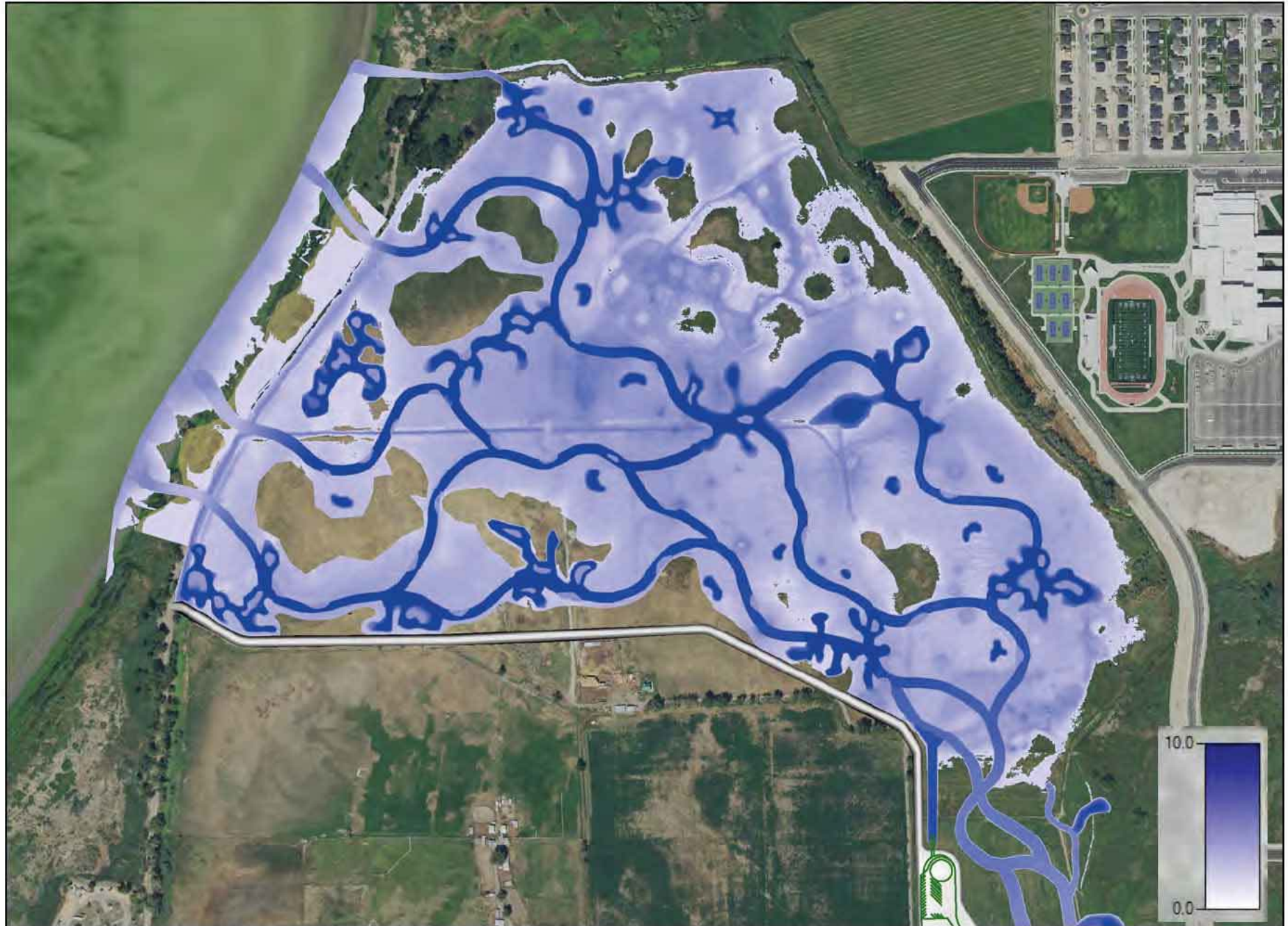
Figure 21. Map of typical variation and complexity in water depth within the "Delta Zone", based on the proposed design. The maximum depth in the delta is somewhat dependant on river discharge and lake level, but is typically between 7 and 10 feet. Page 71 of 111
