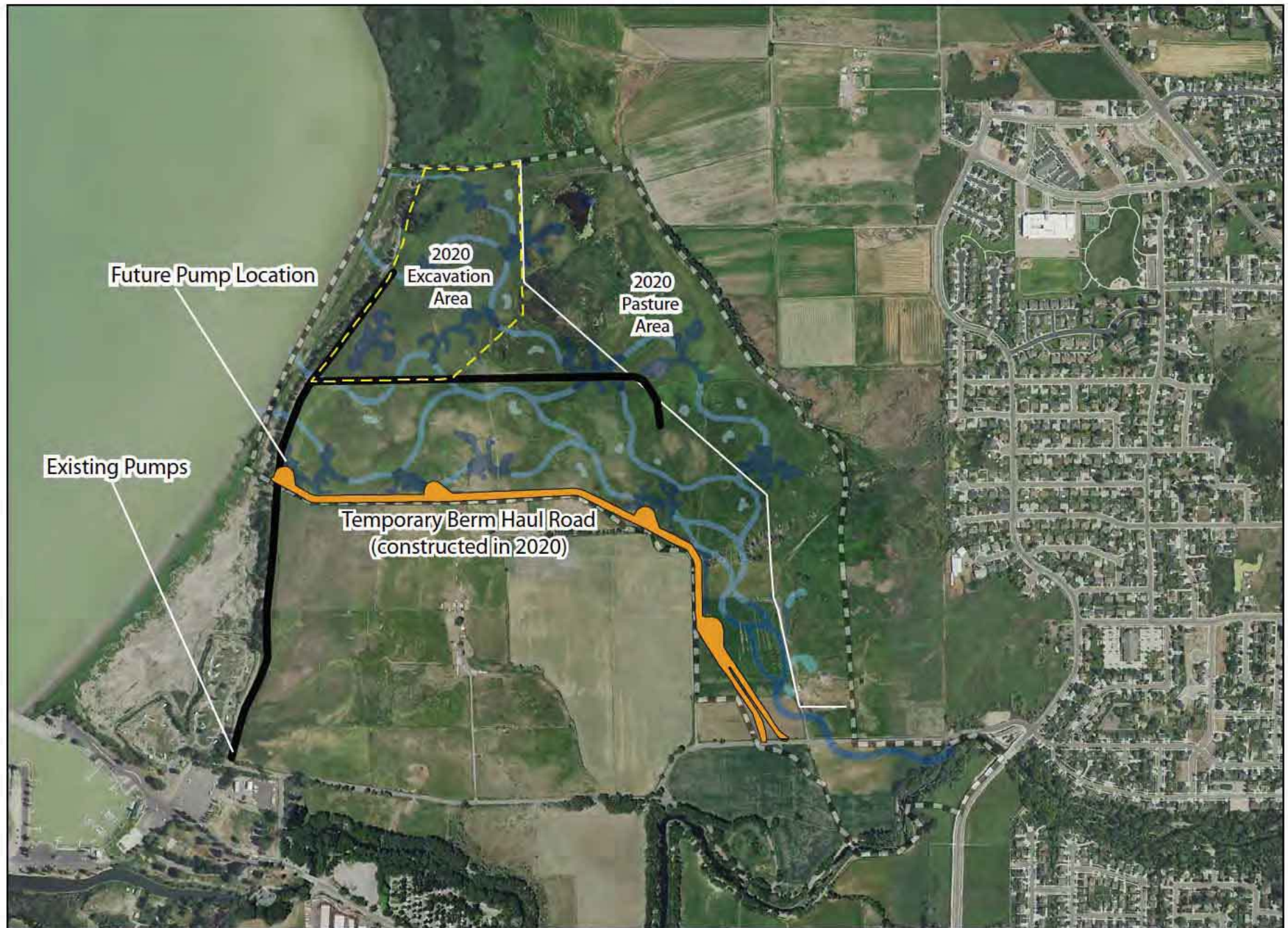
Figure 59. Map showing existing major drainage ditches (black) that route water to the existing pumps. A new pumping location will be established in the general area indicated. The estimated area of 2020 excavation is outlined in yellow, as is the location of a future temporary fence (white line) that will create a pasture to the east where the former owner will be allowed to graze cattle in 2020.
