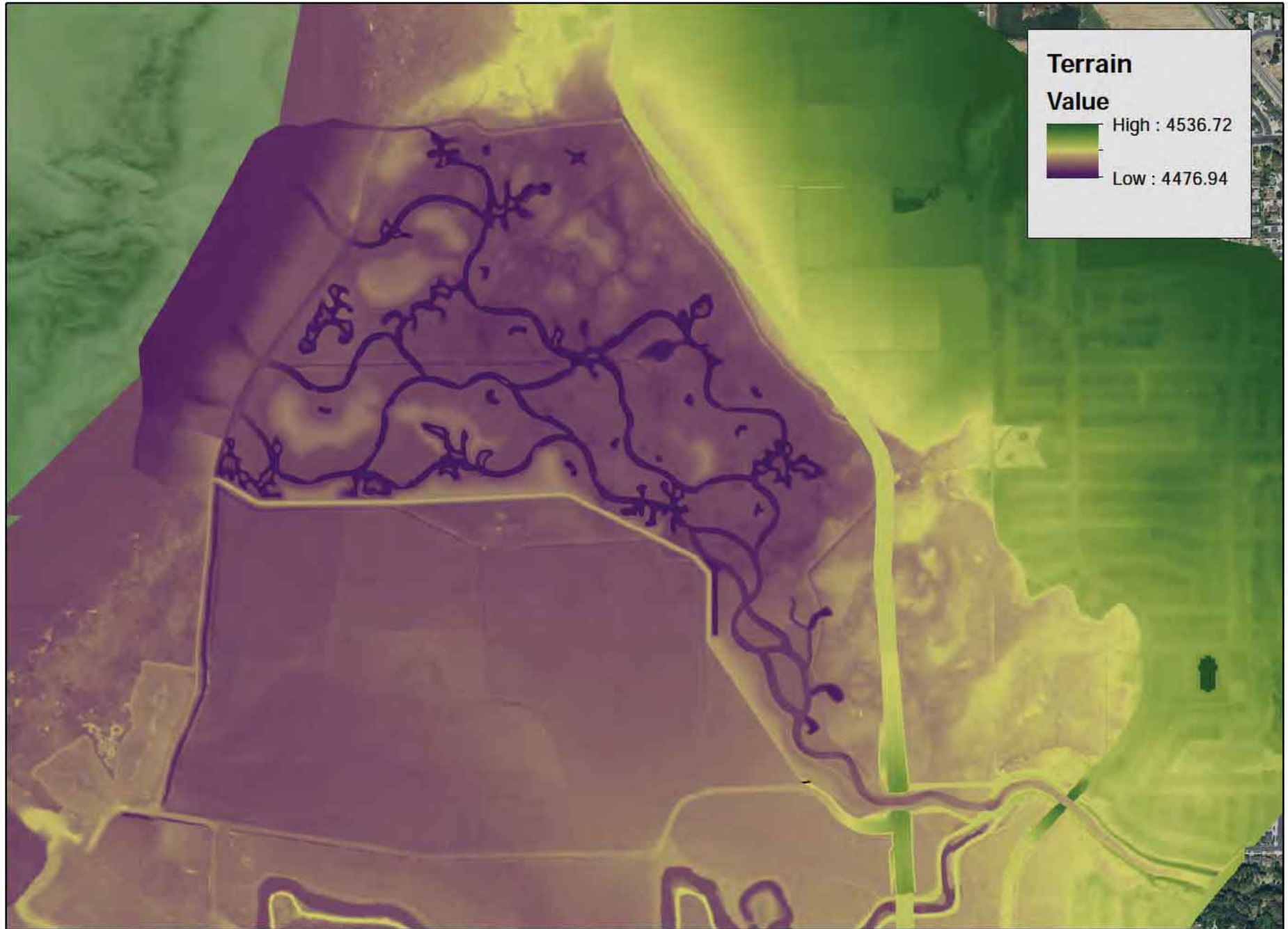
Figure 49. Terrain model of design features used for the current round of two-dimensional HEC-RAS modeling.
